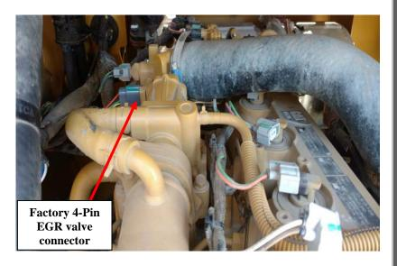
6) Remove the factory 4- Pin Female connector located on the engine harness from the EGR Valve. Press and release the locking tab to disconnect.
