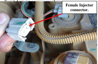
3) On the module harness, the female connectors will connect to each individual injector. Injector connector **A** will connect to the injector closest to the flywheel. They will then connect in order with connector **D** ending on the injector closest to the fan/serpentine belt.
