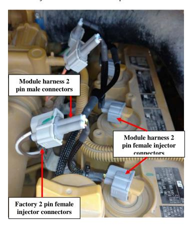
4) On the module harness, now connect the male two pin connectors to the female injector connectors from the factory engine harness. Repeat the initial order by going from connectors **D** through **A**.
