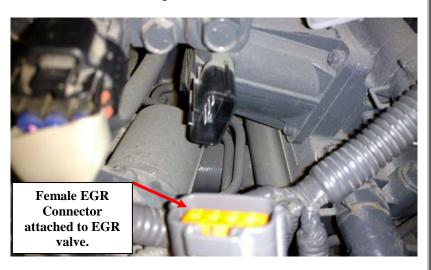
7) Insert the 4-Pin Female Connector from the module harness into EGR Valve. Insure that the connector latch is on the ramp side of the sensor.
