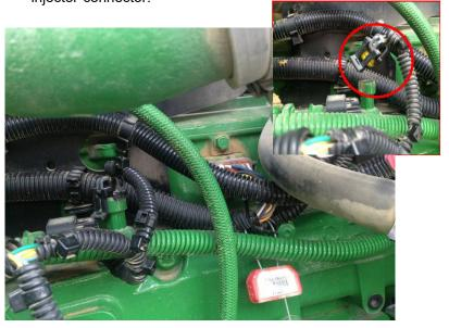
6) Check inside the MAP sensor located on the air intake for a plastic insert. If there is a plastic insert, you will need to remove it and place it over the stock MAP sensor connector that you removed in Step 5.
