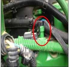
Route the red power wire with the ring terminal to 8) the alternator. Connect the red wire to +12 volts. Connect the black wire with the ring terminal to Ground.
