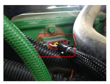
**4)** Plug in the stock male injector connector that was removed in Step 2, to the female injector connector from the module.
