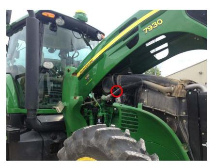
2) Remove the stock injector connector from the engine head. Squeeze the release tabs on each side together to
