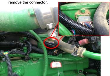
**3)** Plug the male connector from the module into the stock female connector on the engine head.
