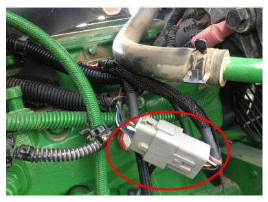
5) Locate the MAP sensor and unplug. It is on the same side of the engine as the air intake and near the injector connector.
