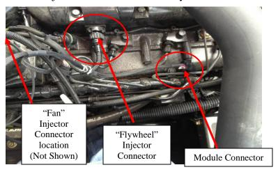
4) On the new harness, the female Injector Connector located closest to the Module will plug into the "Flywheel" Injector Connector on the engine head. The female Injector Connector located furthest from the Module will plug into the "Fan" Connector on the engine head. The Male connectors plug into the Stock Injector Plugs removed in Step 2.
