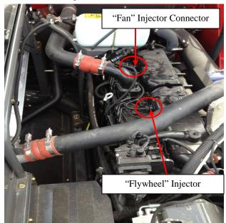
2) Disconnect both Fan and Flywheel plugs. Rotate the outer collar of the injector connectors counter-clockwise to loosen from the side of the engine
