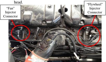
3) Facing the side of the engine, route the Module Harness as shown in the pictures below. The Module Connector will be located to the Right of the Injector Connector labeled "Flywheel".
